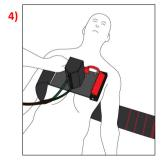
Make sure not to place the piston foot to far down towards the tip of the sternum or too high up on the chest. This could cause injury to the patient or/and cause insufficient compressions.
