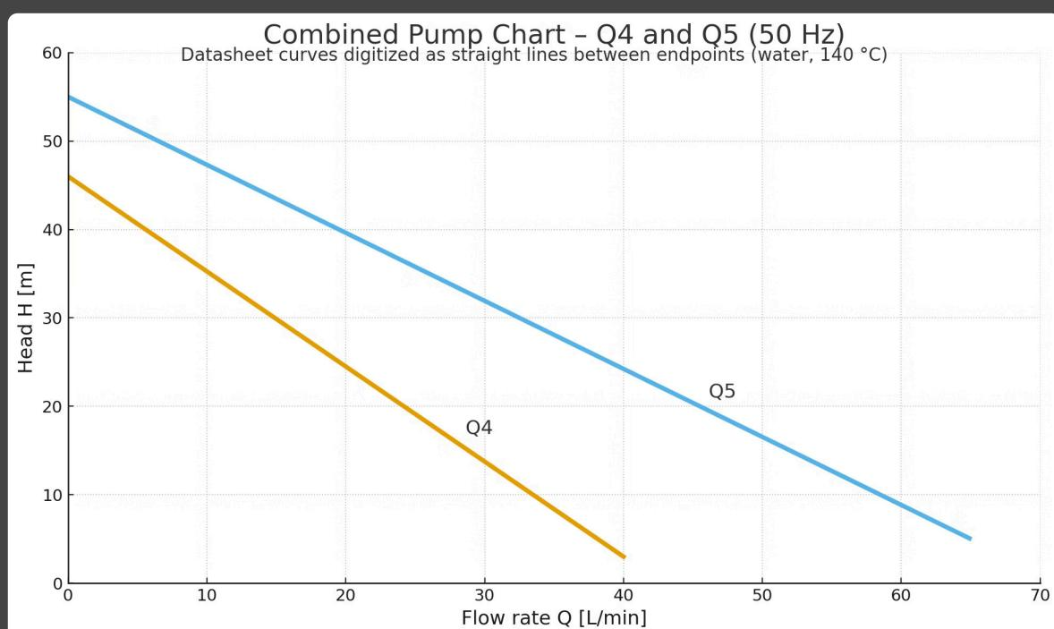
**Nominal duty points:** **Q4:** 20 L/min at 2,5 bar | **Q5:** 45 L/min at 2,0 bar
