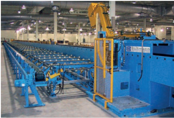
1-fach-Stangenziehanlage für Supraleitermaterial Single bar drawing line for superconducting material
