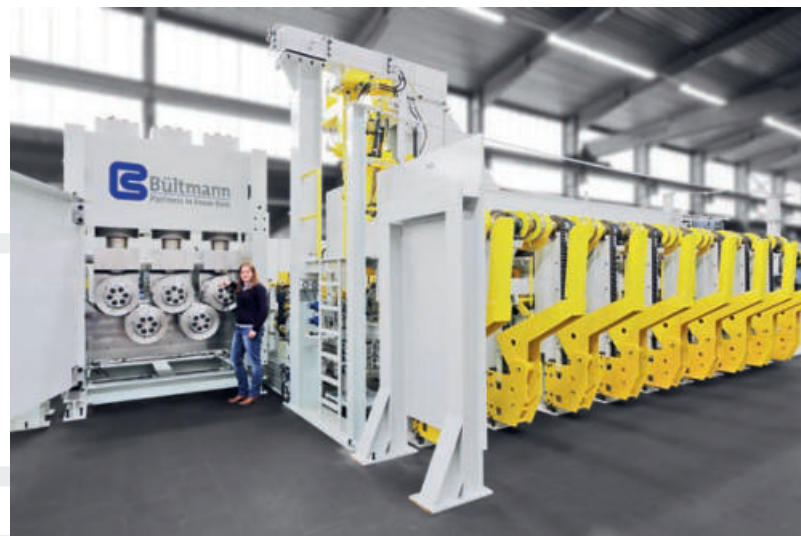
5-Rollen-Vorrichtmaschine für Stahlstangen 5-roll pre-straightening machine for steel bars
