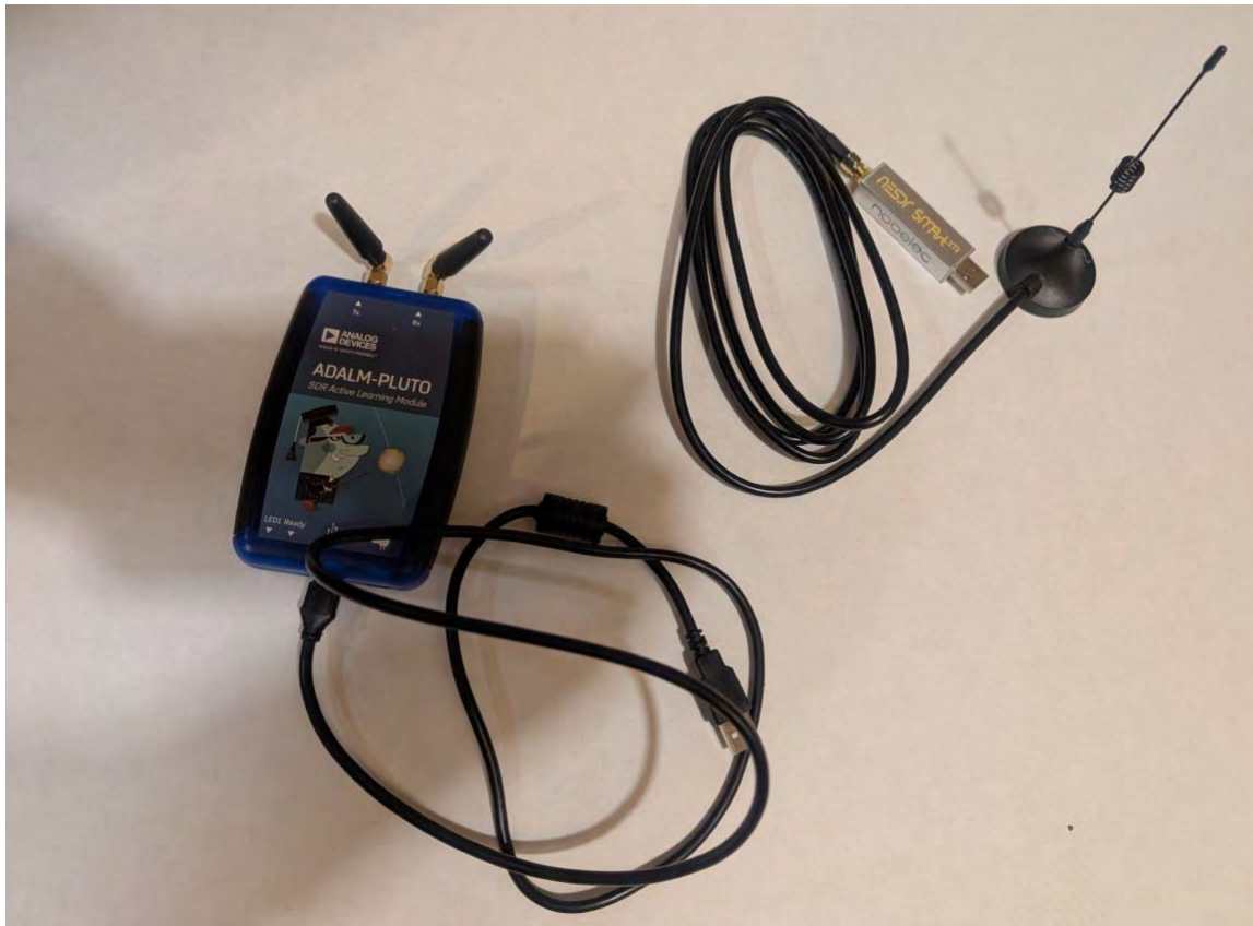
Figure 7.1 Software Defined Radios (ADALM-PLUTO and (Nooelec NESDR Smart XTR)
