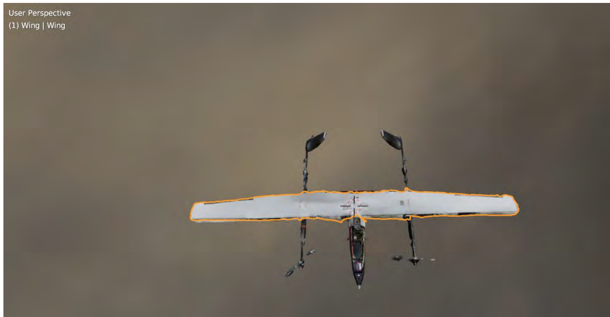
Figure III.6 3d Model of the SuperVolo in Blender, Generated with Polycam
