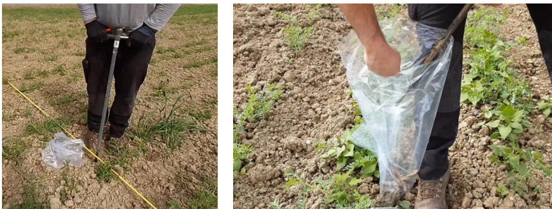
Figure 10: a) Soil probe is inserted up to 30 cm in the mineral soil. b) the soil sample is divided into two pre-labelled plastic bags for the 0-10 cm and 10-30 cm composite samples. Photo credit: Patricia Gallejones.
