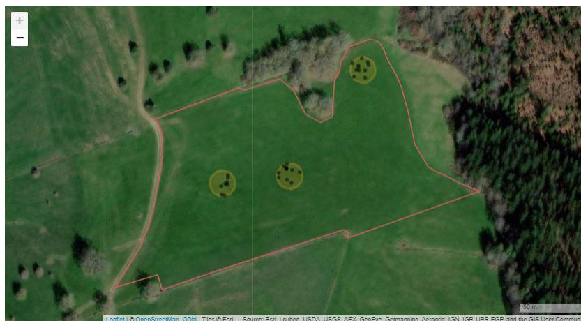
Figure 3: Two-stage stratified random sampling from geographical compact strata. a) The first stage consists in dividing the area of interest into equal-area compact strata and selecting one point per stratum randomly. b) The second stage consists of delineating plots of 10 m radius around the locations and selecting randomly 10 points per plot. The area of interest is a pasture at Behialde (Bizkaia, Spain).
