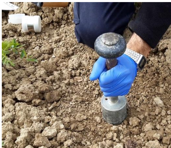
Figure 12: The metallic ring has an adapter holding device (a piston) to facilitate sampling for bulk density. Photo credit: Patricia Gallejones.
