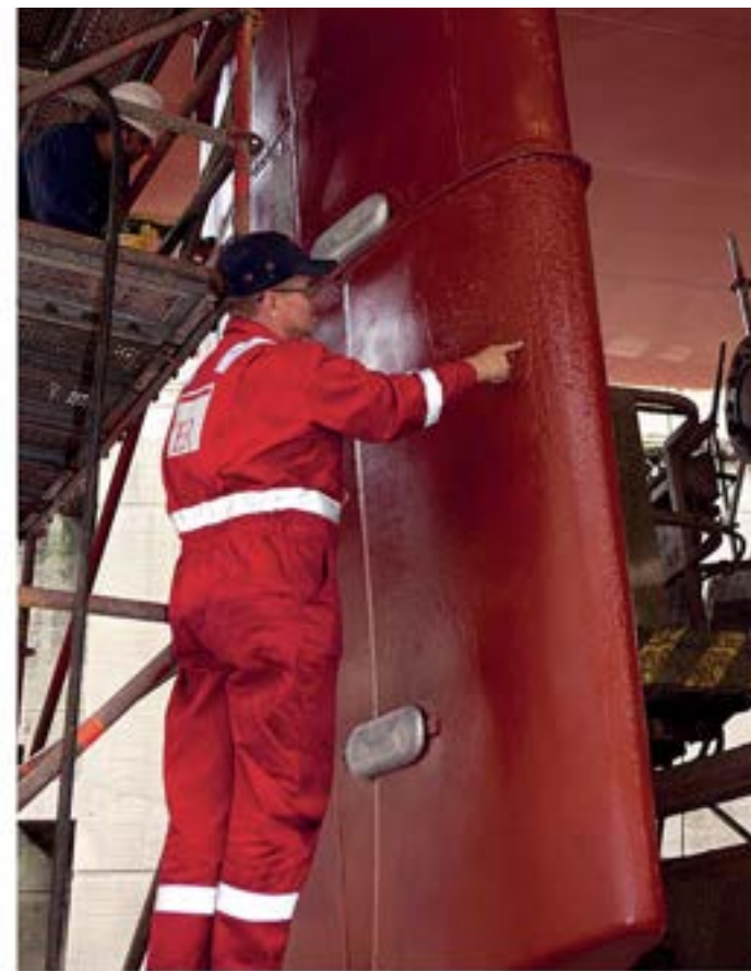
The same rudder 7 years after the original Ecoshield application. No repair of the rudder has been done during that time. No recoating with Ecoshield was needed. The rudder showed no further cavitation damage in that time. (It has been repainted for cosmetic reasons only.)
