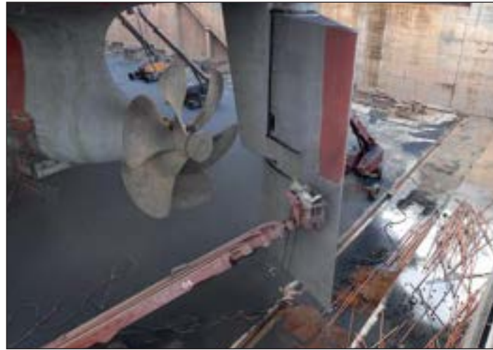
Surface preparation of a rudder prior to application.
