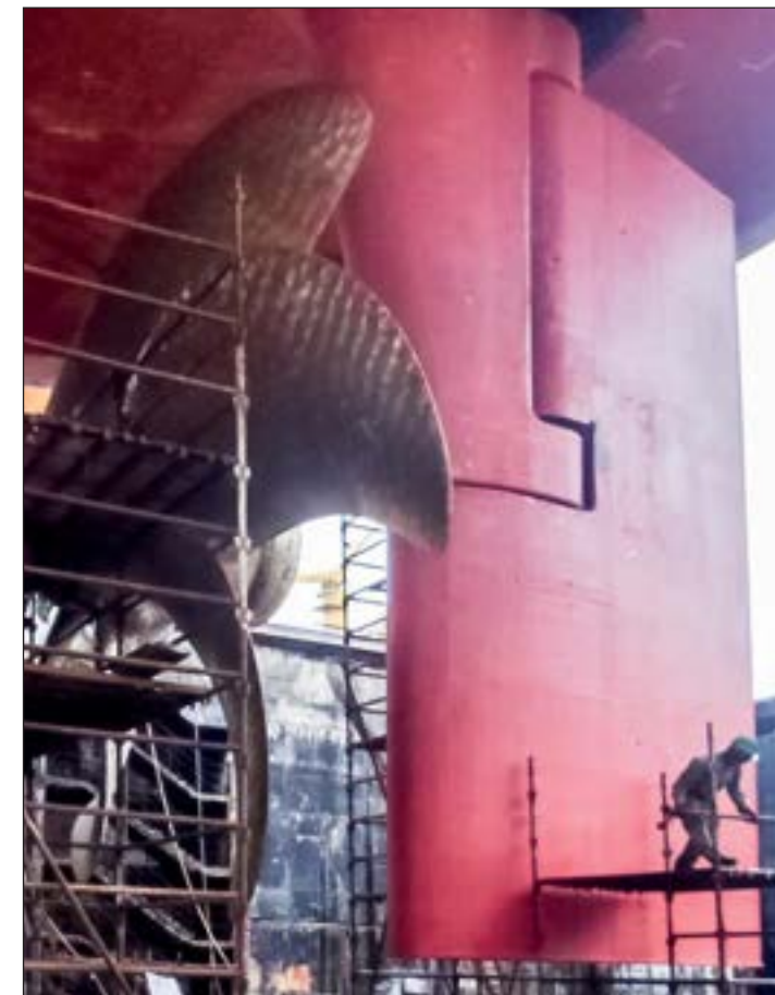
Rudder of m/v Deva after five years of service with Ecoshield.
