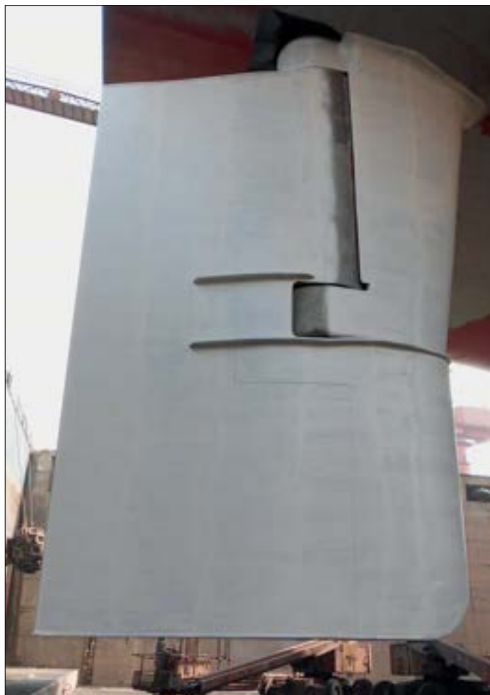
Ecoshield is applied in two identical layers. Rudder with first layer of Ecoshield (left) and after second coat (right). Different colors are used to make it easy to detect gaps or holidays in the second coat.
