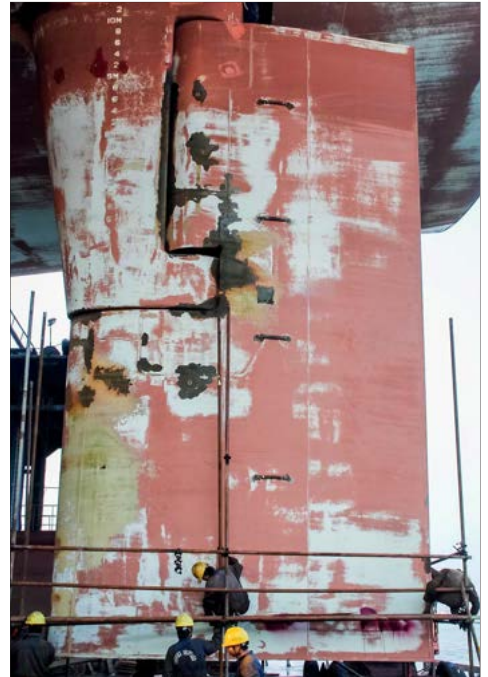
The rudder of m/v Deva when the vessel came into drydock five years ago, showing multiple damages.
