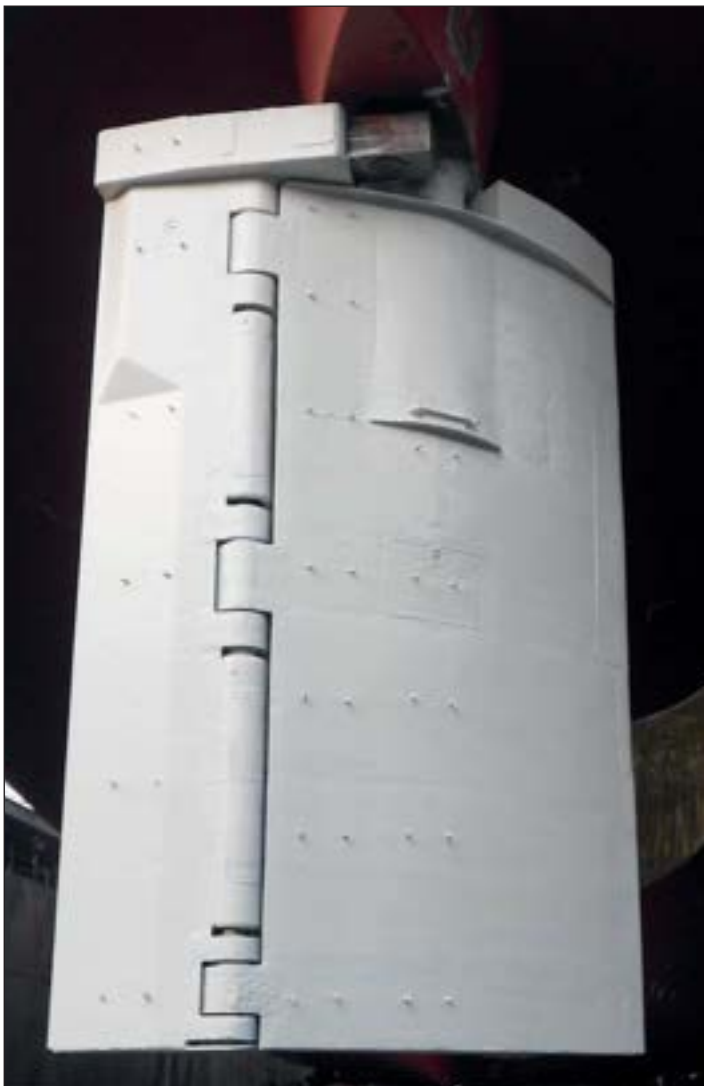
Ecoshield will protect a rudder against cavitation damage.
