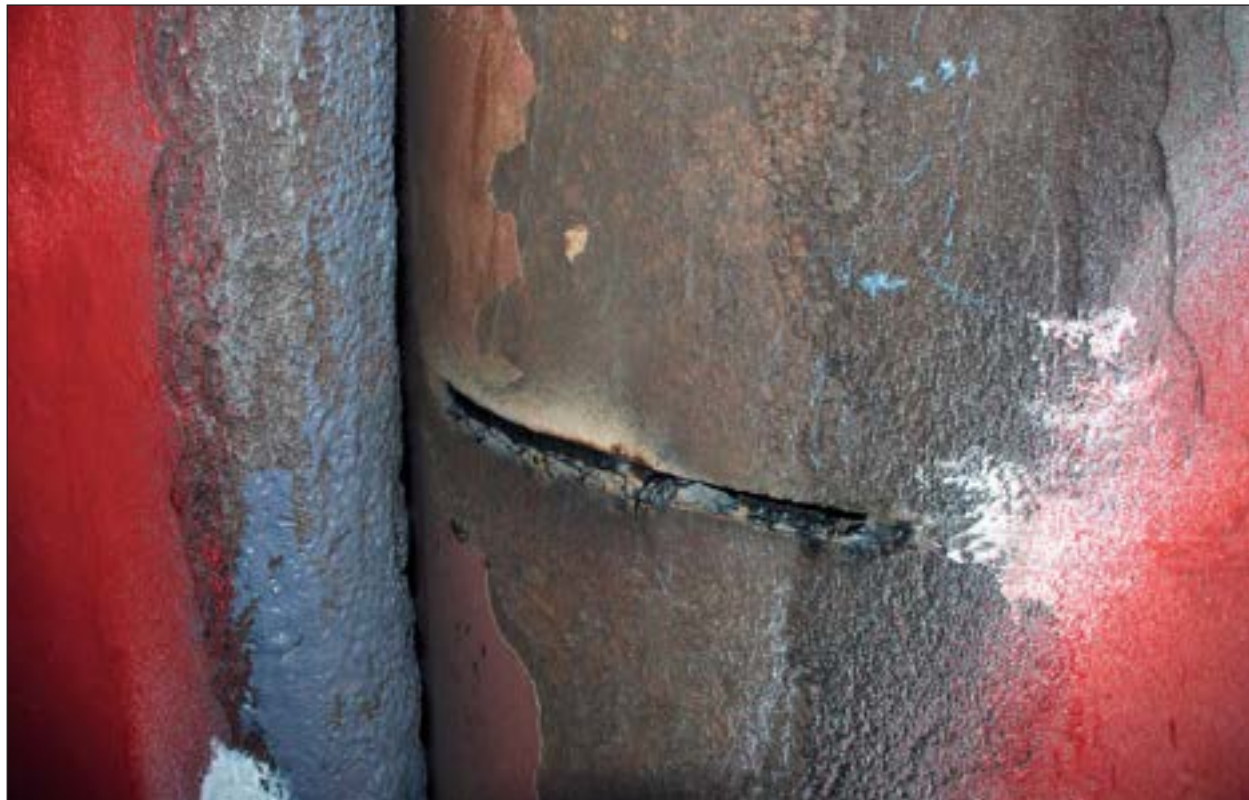
Severe cavitation damage on the rudder prior to Ecoshield application.
