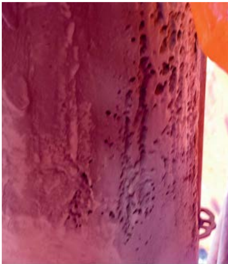
State of rudder of ro-ro ship in 5 years after it was built in 1999. The rudder was blasted and coated with Ecoshield (then Ecospeed) in 2004. Due to time constraints the pitting was not repaired before application.
