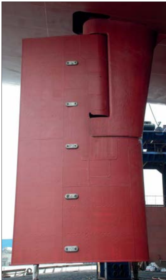
Ecoshield was applied in 2009, protecting the rudder from then on.
