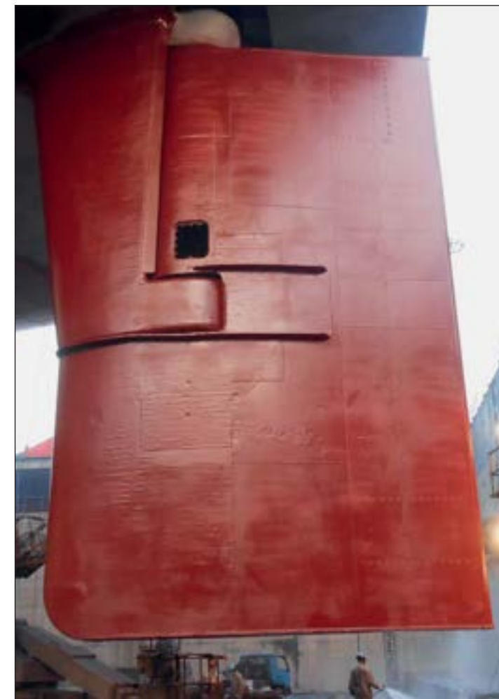
Ecoshield is applied in two identical layers. Rudder with first layer of Ecoshield (left) and after second coat (right). Different colors are used to make it easy to detect gaps or holidays in the second coat.
