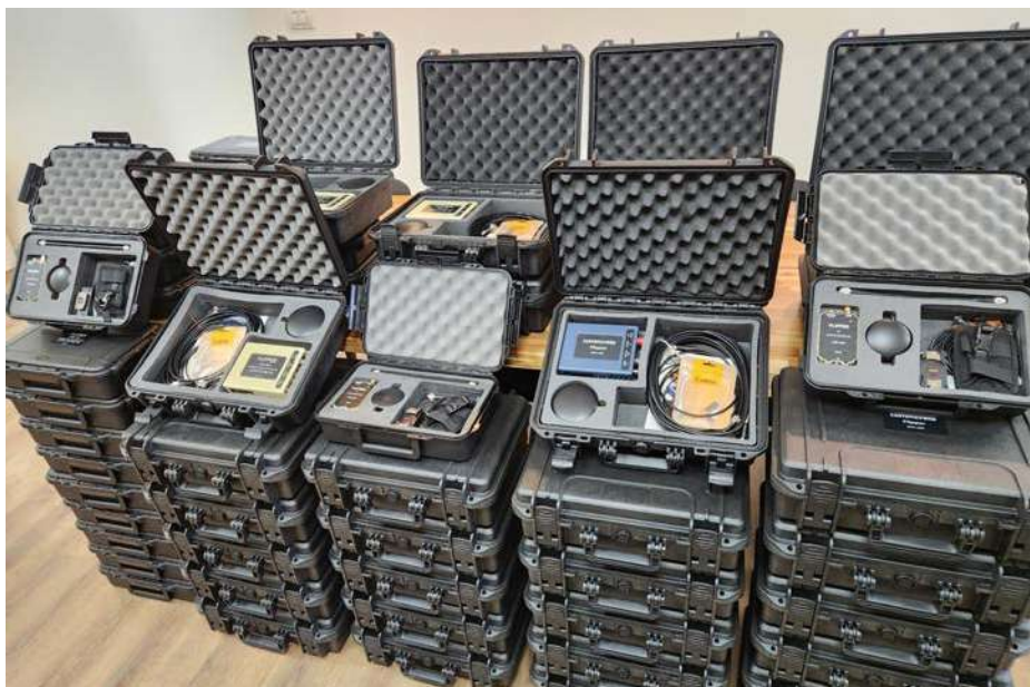
Commcrete equipment kits prepared for operational deployment. Multiple Pelican cases contain complete Commcrete systems ready for fielding across different mission sets. Each case houses antennas, cabling, power supplies, spare batteries and configuration documentation tailored to specific user profiles and operational theatres. This staging photograph underscores the company's emphasis on rapid deployment and unit-level self-sufficiency, allowing teams to unpack, configure and activate satcom connectivity within minutes of arrival at an operational location.
