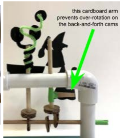
clear PVC tubing keeps the dowel and cams in place
