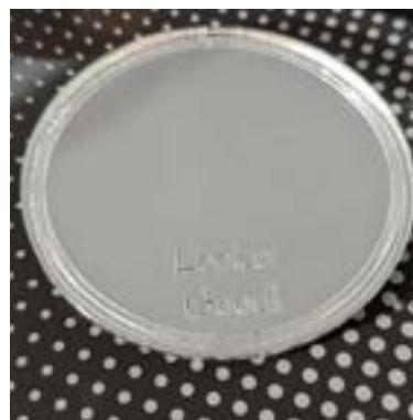
Text and designs must be flipped before being engraved into the back of mirrored acrylic
