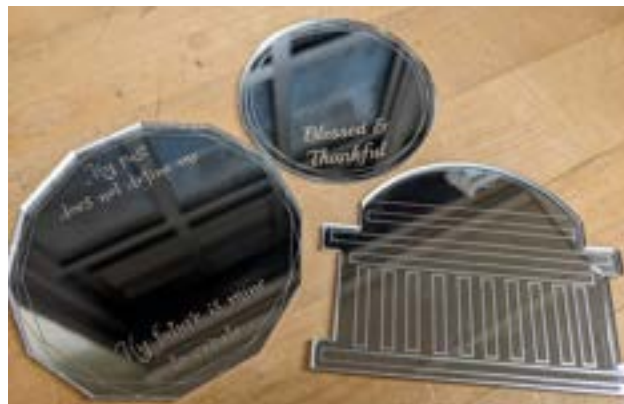
Examples of a Cut, Score, and Engrave: the three types of operations available on laser cutters
