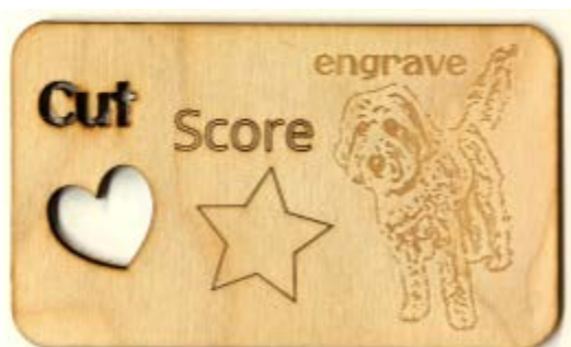
Examples of a Cut, Score, and Engrave: the three types of operations available on laser cutters
