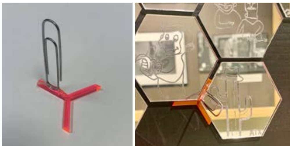
Laser cut spacer used to evenly arrange tiles
