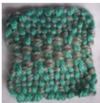
Sample showing Plain Weave (top) -- Basket Weave (middle) -- Plain Weave (bottom)
