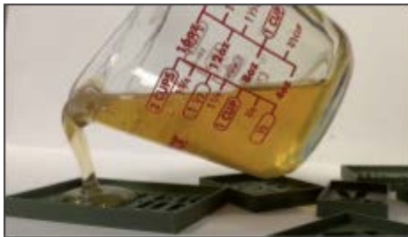
Pouring the melted rubber from a microwave safe dish into 3D printed molds
