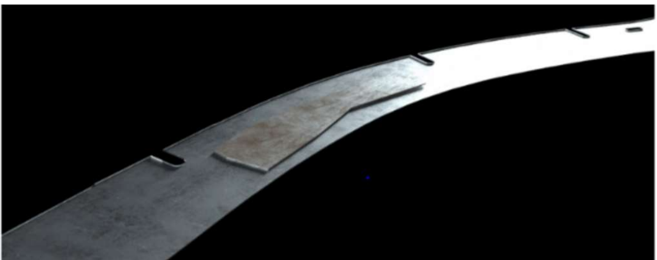
An example of a patched blank before stamping
