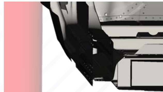
65 ms: Max. deformation, no contact with battery modules
