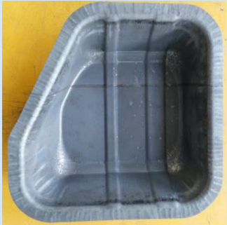
The samples replicate a corner of a battery tub design
