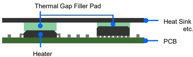
In areas where space between surface is uneven or varies and where surface textures are a concern regarding efficient thermal transfer, the supple consistency of Gap Filler Pad is excellent for filling air gaps and uneven surfaces.
