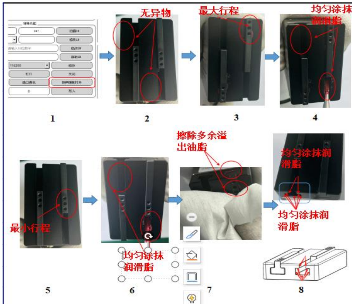
Figure 11.2 Grease maintenance flow chart
