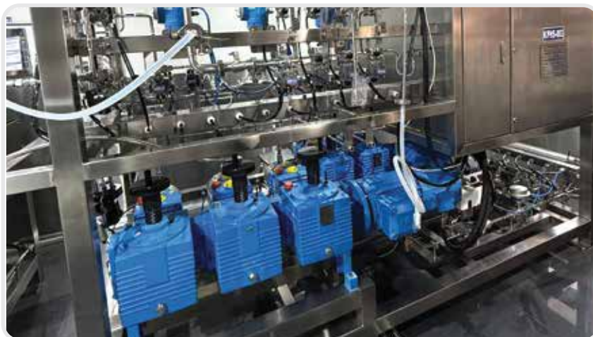
Preparative HPLC systems - 3 L/Min and 8 L/min (with 200 & 450 mm DAC Column)
