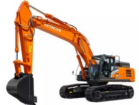
Hitachi ZX350LC-5 33t Excavator
