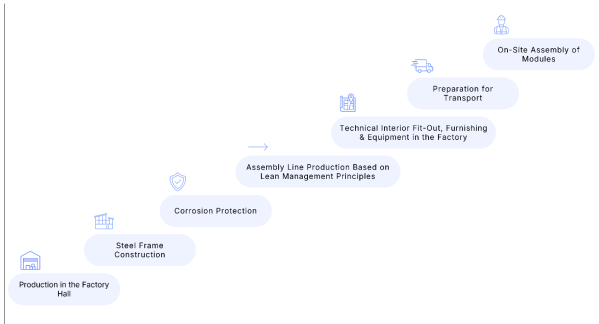
Figure 1: Process Flow of Modular Construction
