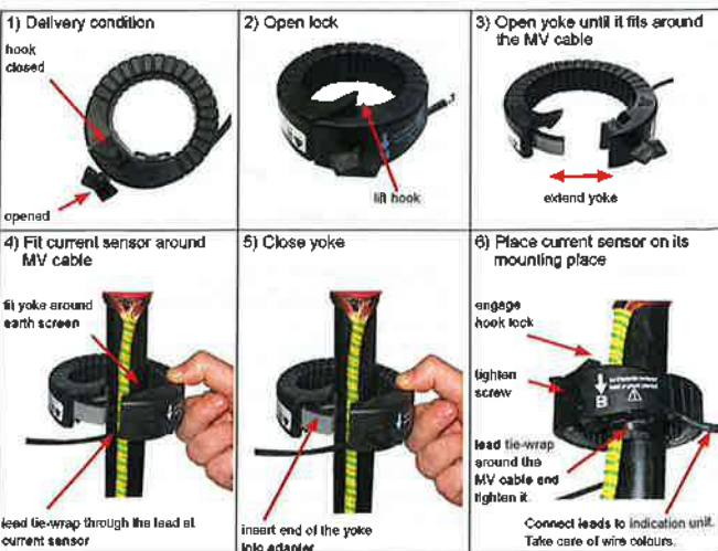
Fig. 3.2: Installation of single-phase current sensors
