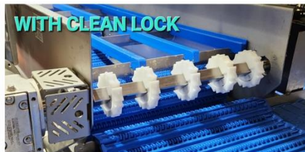
CleanLock sprockets installed 2 years ago. No sign of wear and no belt damage observed since.
