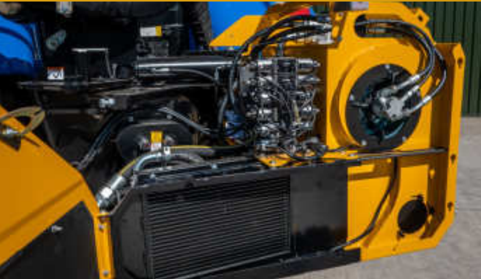
Integrated Oil Cooler
