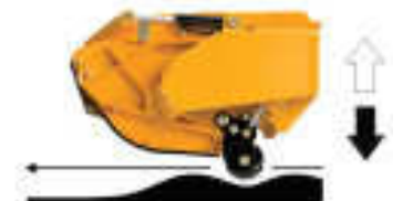
Lift float OFF
