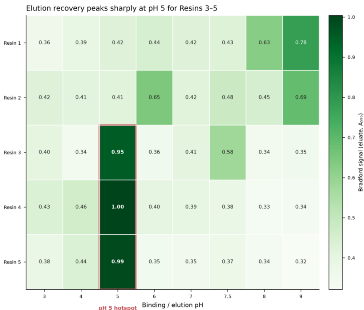
Figure 5. A single run localizes the optimum. Bradford signal for the eluate of each resin × pH combination. A sharp recovery hotspot emerges at **pH 5 for Resins 3, 4, and 5** (signals of 0.95, 1.00, and 0.99 respectively) — roughly 2–2.5× the background seen across most other conditions. The pattern is unambiguous and would have required 40 separate column runs to establish conventionally.
