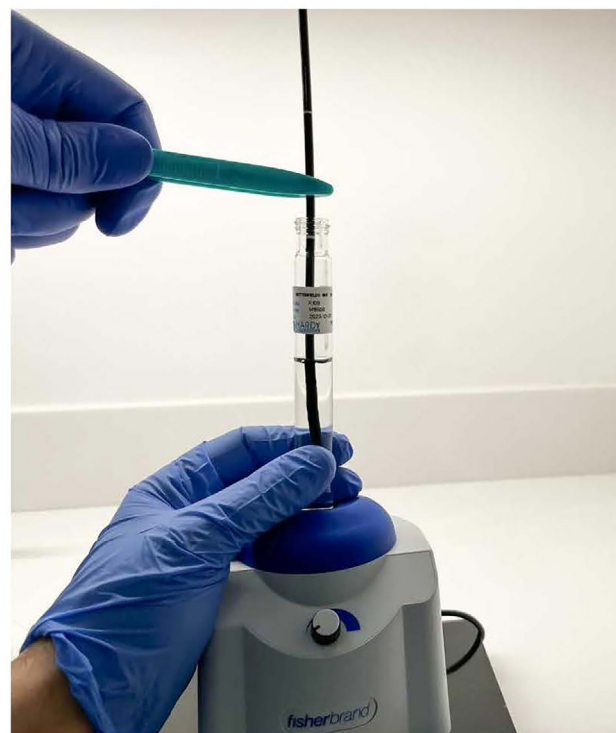
Fig. 2. Sample collection from the flexible fiberoptic laryngoscope (FFL) distal tip surface using vortex and collection tube. [Color figure can be viewed in the online issue, which is available at www.laryngoscope.com .]
