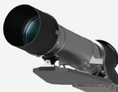
OPT 120 A 1 m Multispectral, Wide Swath Imager • Designed for Large Area Coverage • 65 km Swath • 9 bands (Red, Green, Blue, PAN, Red Edge-1, Red Edge-2, NIR, NNIR) • Currently at TRL 6
