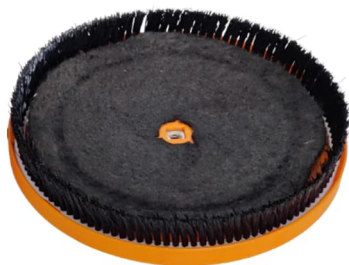
Protective felt defective, must be replaced
