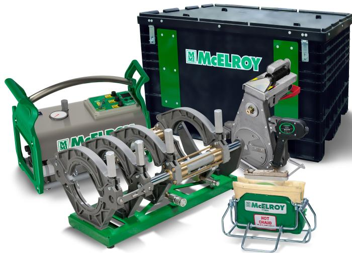
The Acrobat 160 is a low-force fusion machine that allows operators to butt fuse pipe in tight work spaces. With its small footprint and optimal weight, it is an easy machine to manipulate when performing overhead fusions in tight spaces as well as on the ground.
