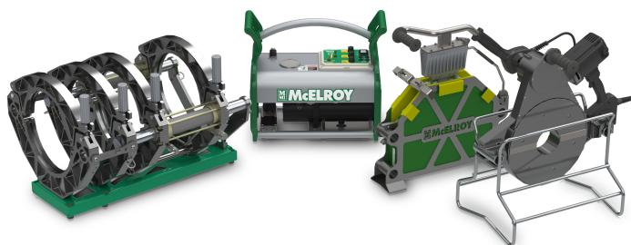
The Acrobat™ 315 fusion machine has a lightweight, compact design for easy maneuvering in tight indoor workspaces specific to the polypropylene industry. To further reduce its footprint, the carriage can be configured from 4 to 3 jaws without tools. A single-size insert design can accommodate a variety of pipe sizes, and its narrow jaws allow fusions to most flanges and fittings.
