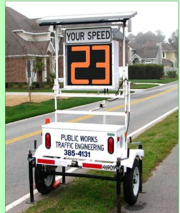
Speed Trailer used in Traffic Calming Program
