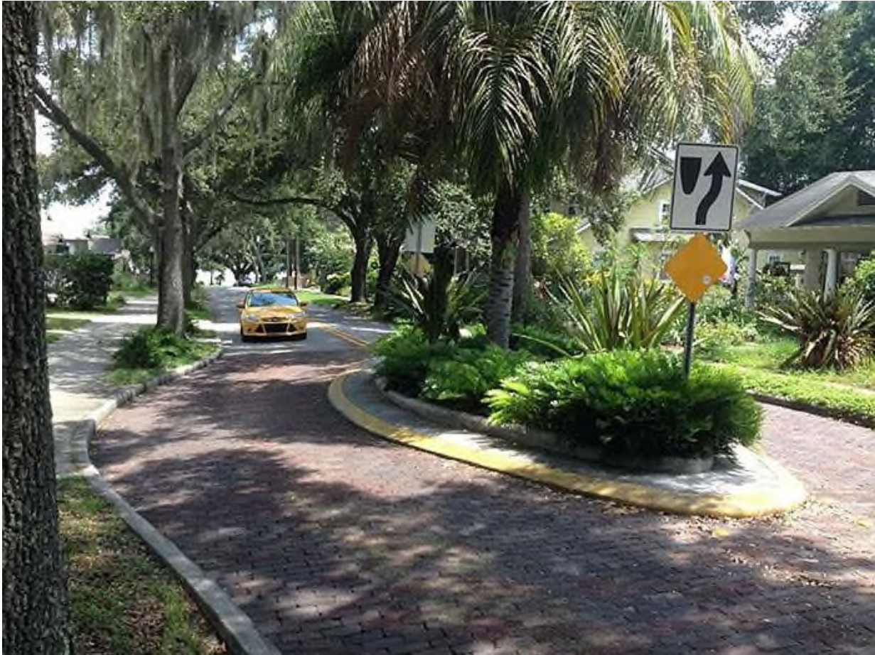
Figure 3.3. Street Width Reduction Measure - Median Island (Source: FHWA Module 1-Ken Sides)
