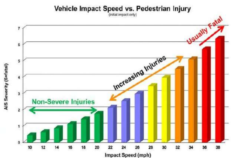
Figure 2.1. Speed/Pedestrian Injury Severity Correlation (Source: FHWA Module 2-C. E. "Rick" Chellman)
