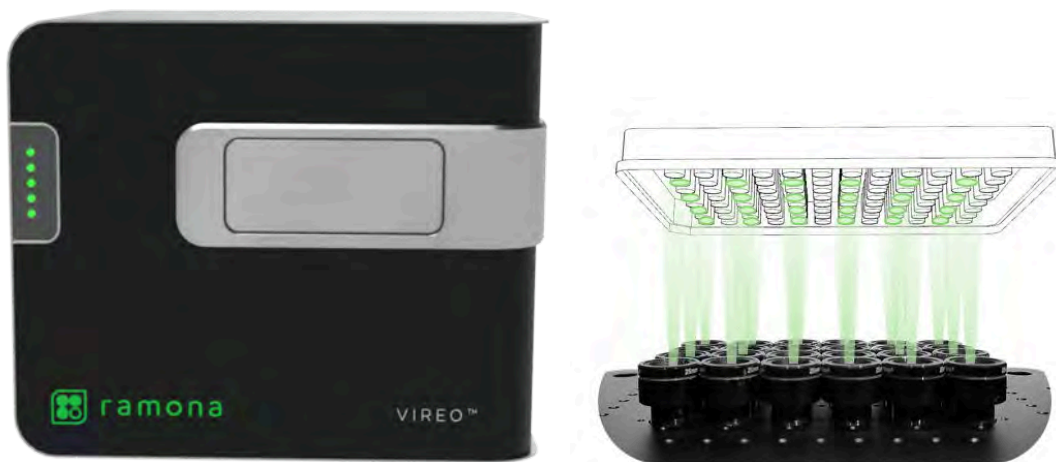
Figure 1. The Vireo (left) features a 6×4 Multi-Camera Array Microscope (MCAM) mounted on a movable platform, enabling rapid imaging of entire well plates (right)
