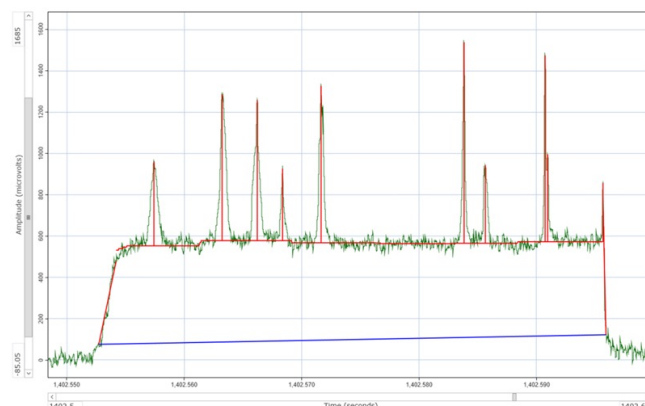
Figure 6: The OhmX platform achieves a high signal-to-noise ratio (in the above case SNR=30) without slowing or stretching the molecule which is traveling up to 1 megabase per second.
