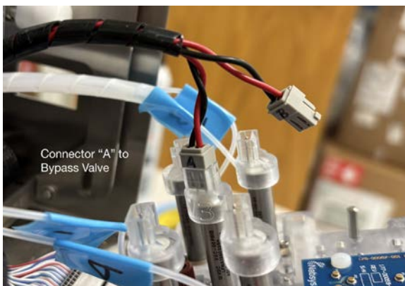
Figure 69: Installing the A connector to the Bypass Valve.
