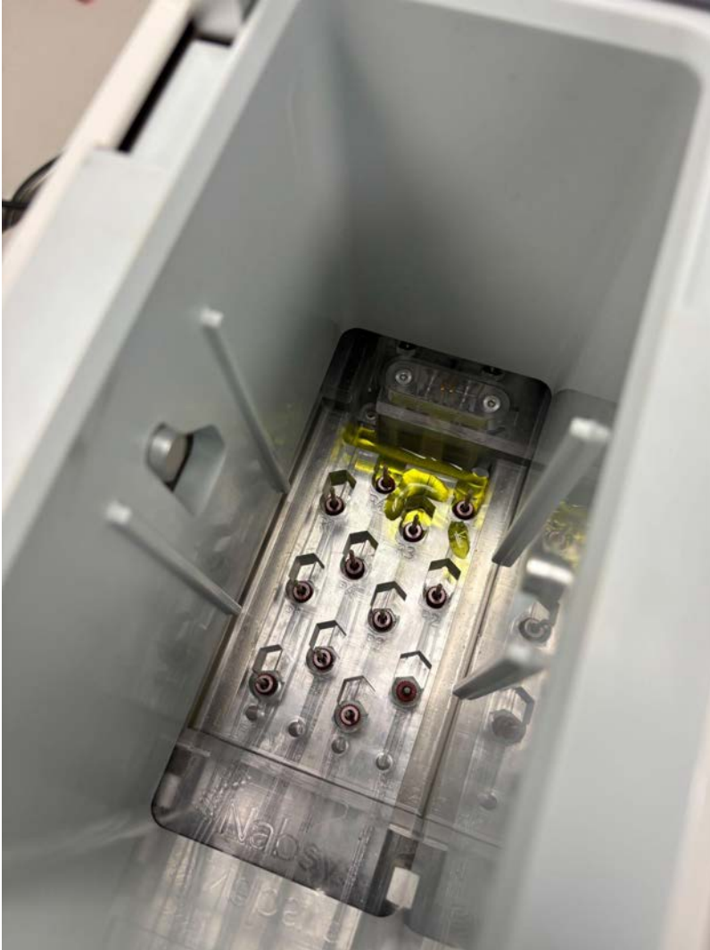
Figure 35: Reagent Manifold with a reagent spill.
