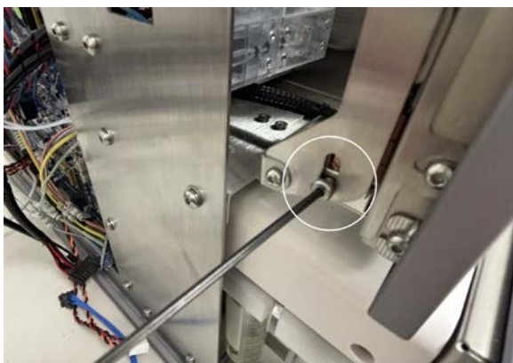
Figure 77: Installing the pivot screws.
