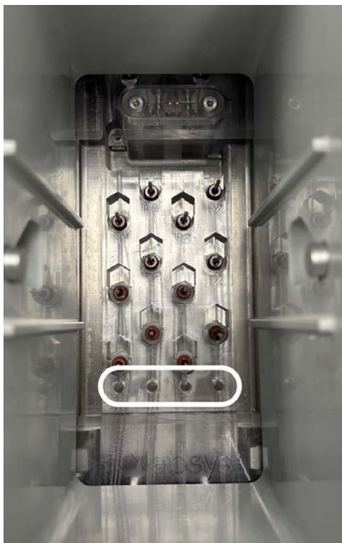
Figure 39: Flushing Reagent Manifold flush ports with syringe and water.
