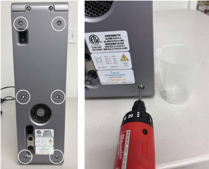
Figure 44: Removing screws from the back panel of the analyzer.
