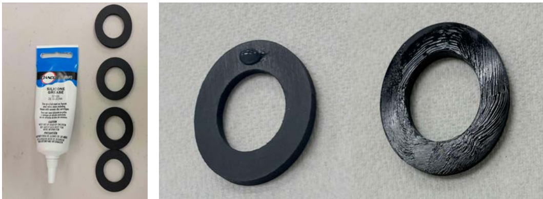
Figure 83: Greasing the waste tube gaskets.
