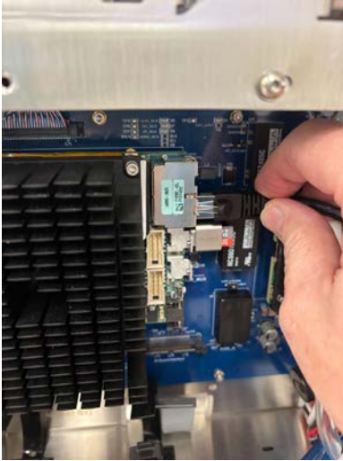
Figure 103: Installing the network cable.
