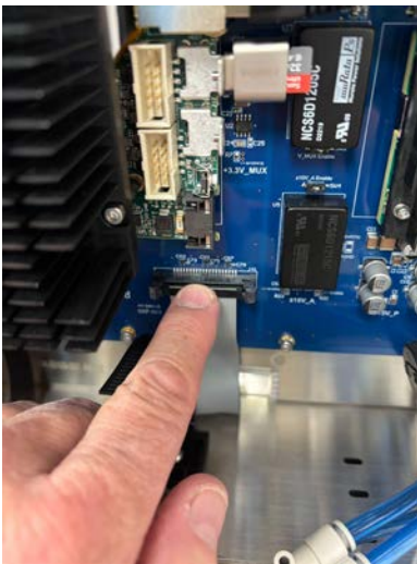
Figure 104: Installing the I/O cable.
