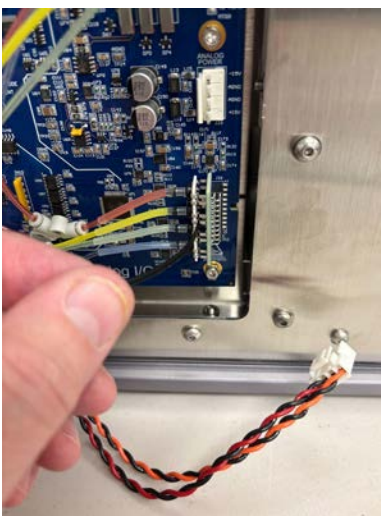
Figure 89: Inserting the bent cable tie in between the transducers and the PCB.
