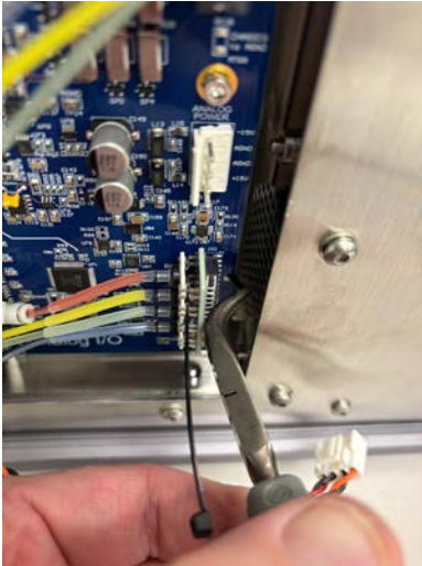
Figure 90: Pulling the cable tie with needle nose pliers.
