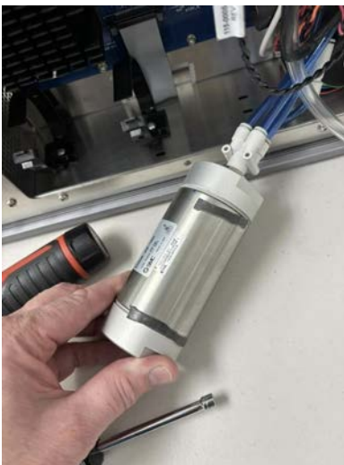
Figure 93: Removing the air storage tank from the straps.
