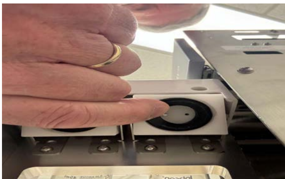
Figure 84: Installing the waste tube gaskets.
