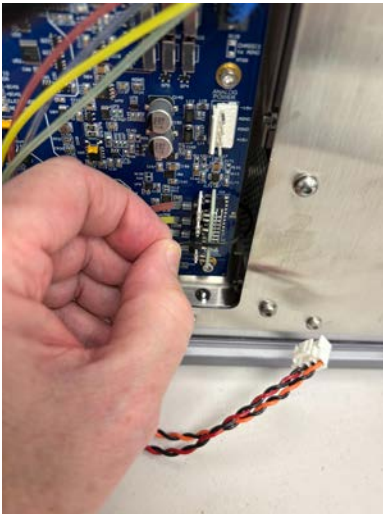
Figure 91: Inserting the tip of the cable tie into the end to tighten.
