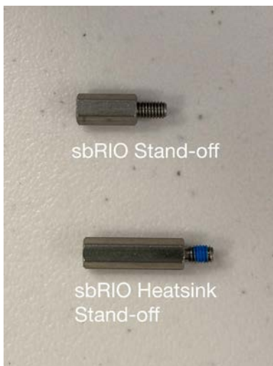
Figure 98: sbRIO (top) and sbRIO heat sink (bottom) standoffs.
