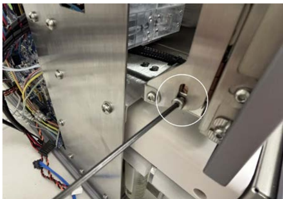
Figure 50: Installing the DAQ pivot screws.
