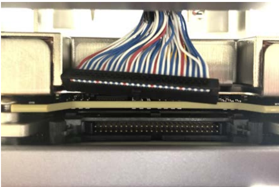
Figure 49: Disconnecting the DAQ Connector.
