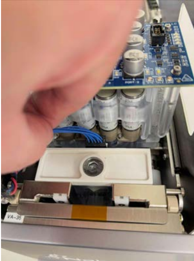
Figure 78: Installing the Electrode PCB cable.
