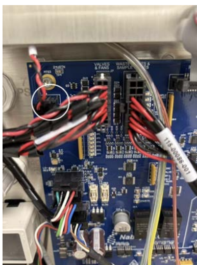
Figure 64: Reconnecting the memory cable.
