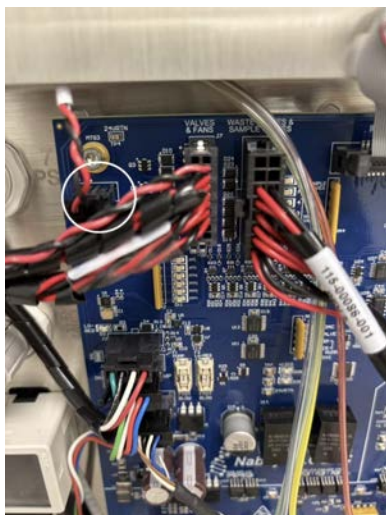
Figure 57: Removing the memory cable on the I/O Control PCB.
