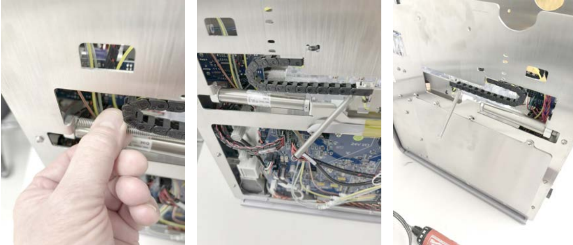
Figure 48: Unhooking the springs on the sides of the detector drawer (left), lefthand spring unhooked (middle), and righthand spring unhooked (right).
