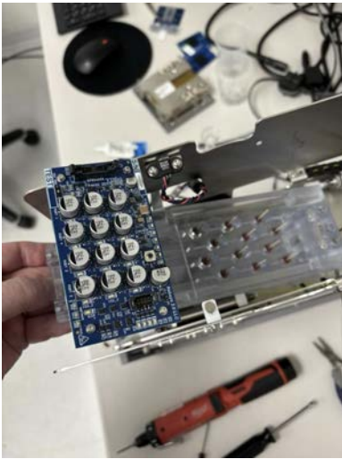
Figure 61: Placing the reagent manifold into the chassis.
