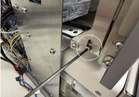
Figure 112: Installing the DAQ screws.
