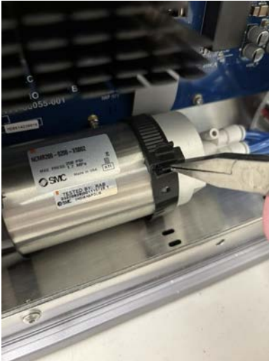
Figure 92: Lifting the locking tab on the air storage tank straps.
