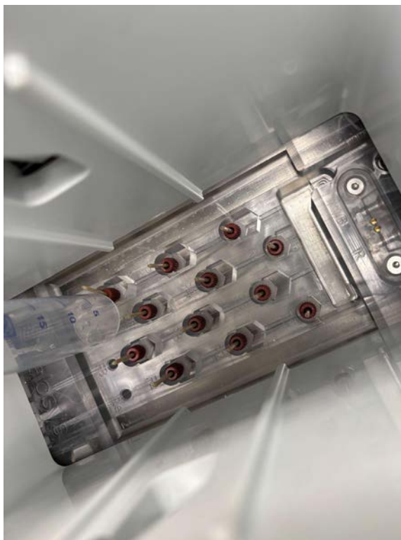
Figure 39: Flushing Reagent Manifold flush ports with syringe and water.
