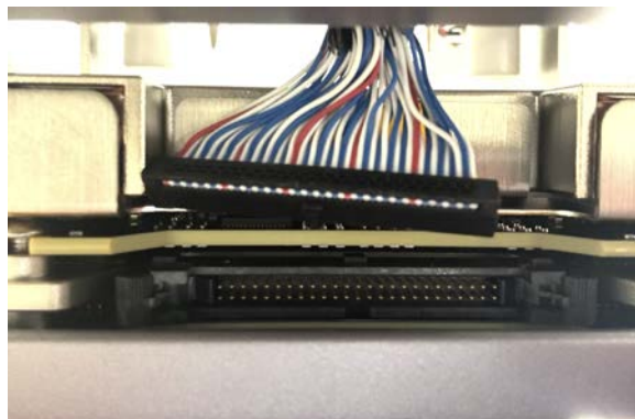
Figure 111: Disconnecting the DAQ cable.
