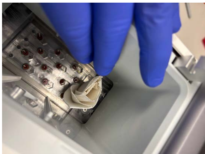
Figure 41: Drying the Reagent Manifold with a folded paper towel.
