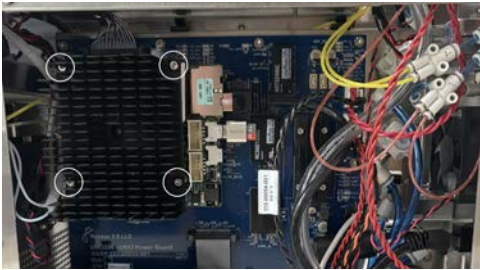
Figure 94: sbRIO heat sink screw locations.
