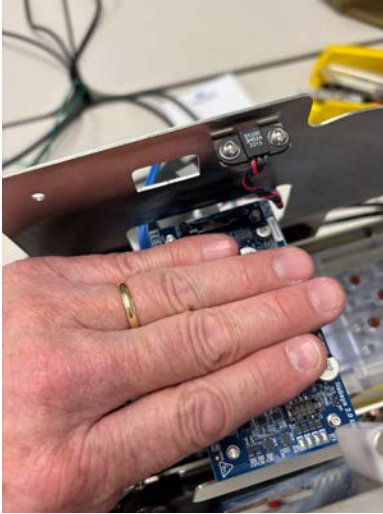
Figure 109: Installing the Pump Control PCB.
