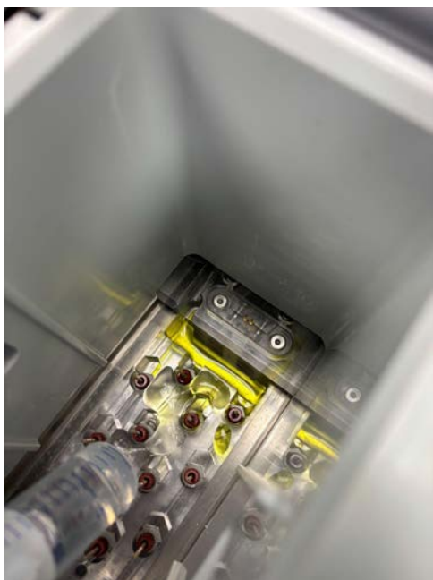
Figure 37: Flushing the Reagent Manifold with a syringe and DI water.
