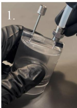
1. Purge from the thin needle at lower position (skip this step when in glovebox)
