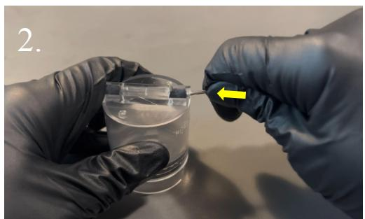
2. Pull both needles out and push in top gaskets to cover the holes
