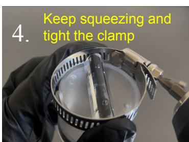
4. Keep squeezing and tight the clamp
