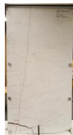
At failure (Push cycle)
