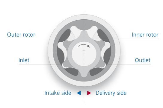
Pumping (clockwise) starts at "6" as space starts to open between the inner and outer gerotors over the inlet (blue) port
