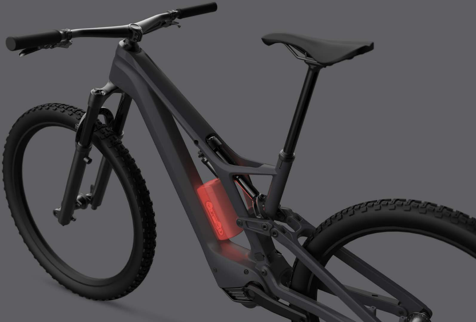
➤ Range Extender: Cilo Light Capacity E-Mountainbikes
