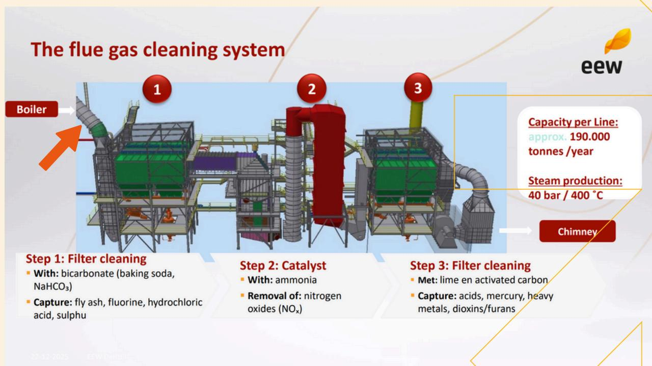
**Important: The proposed technology must be capable of integrating with the existing flue gas cleaning system, preferably at a feed-in point upstream of the current cleaning stages (see orange arrow).**
