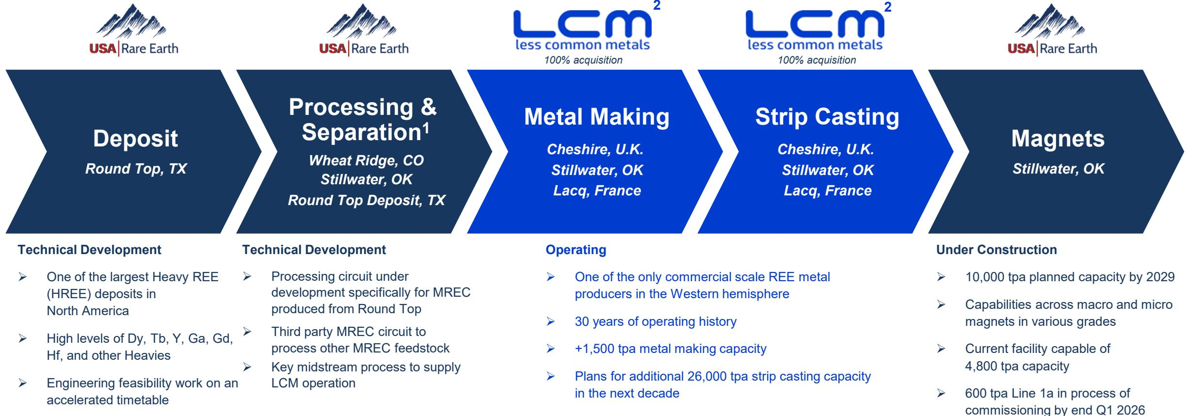
1. Two-stage process: (i) Processing stage to extract rare earth and other critical elements; and (ii) Separation stage to isolate HREEs into individual Rare Earth Oxides (REOs)
