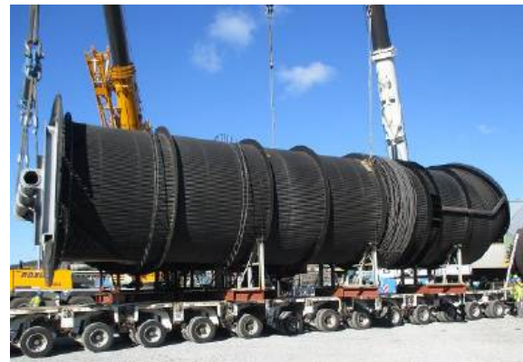
Arcelor Mittal, Europe, 35 – 40 t/h Off-Gas Quantity, max. 180.000 Nm 3 /h
