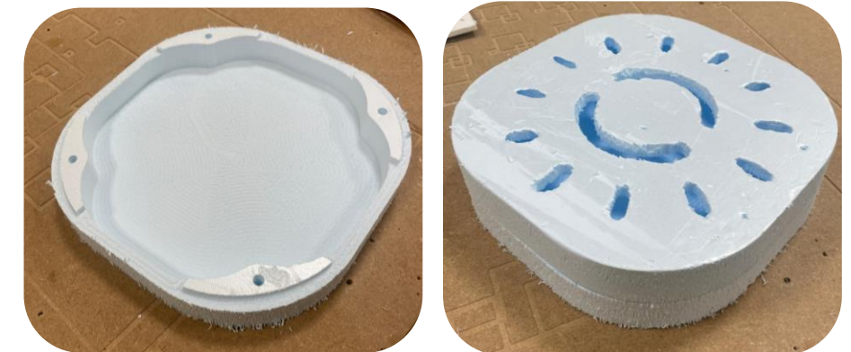
Figure 35 Foam mock-up confirms CAD model
