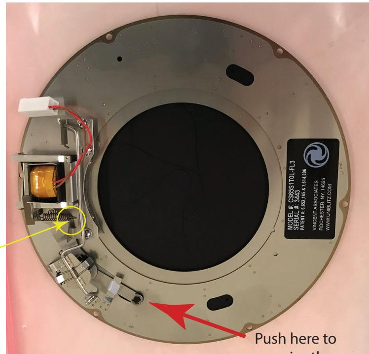
If the shutter fails to close 100%, increase spring tension by gently bending the arm holding the spring toward the center of the shutter.
