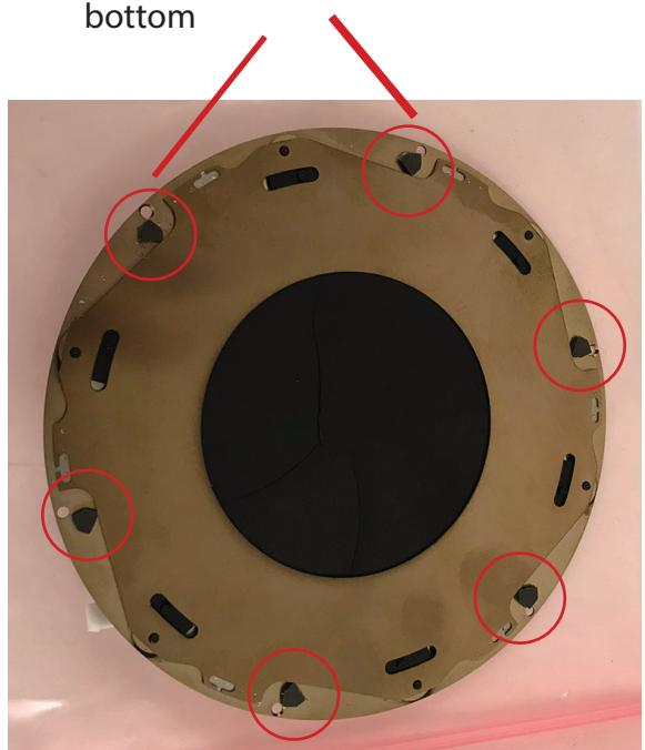
Remove these screws to detach the shutter from the CCD housing. Do not unplug the shutter.
