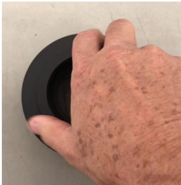
Unscrew the front flange from the Micro-Line camera.
