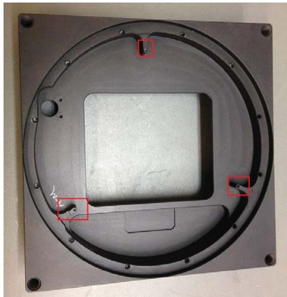
Remove these screws to detach the shutter from the CCD housing. Do not unplug the shutter.
