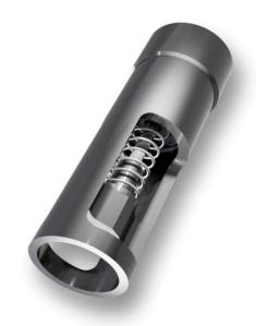
The GS Equalizing Assembly is designed to maintain pressure balance from both above and below when assembled with the S Lock Assembly. The configuration is chosen based on the specific landing profile intended for the plug. Once assembled with the S Lock Assembly, the plug is pinned onto the C-1/C-2 Running Tool and set with wireline in the corresponding profile.
