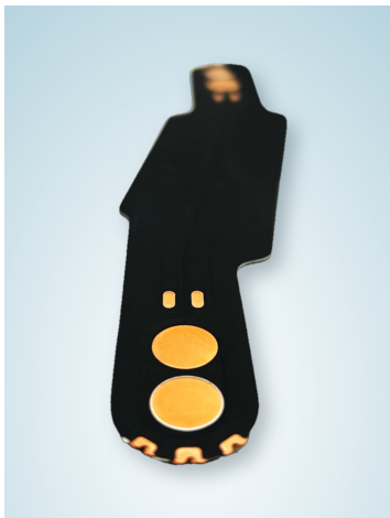
Cellink's incredibly thin flex harness efficiently carries high currents.
