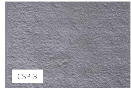
Suitable surface preparation methods are grinding, high-pressure water blasting (at least 350 bar) and sandblasting/shotblasting.
