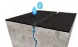
Elastic but not crack bridging: The waterproofing layer does not withstand permanent water pressure.
