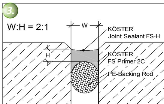
3. The Joint Sealant should be installed so that the ratio of joint height: width corresponds to the norm requirement. A detailed table is provided in the Technical Guideline.
