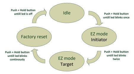
When cycling through the menu modes, the state is indicated by a number of 100ms blinks on the LED. The device is supporting the ZigBee standardized EZ- mode Commissioning.
